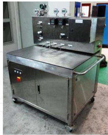
▲ Water Membrane Monitoring System
